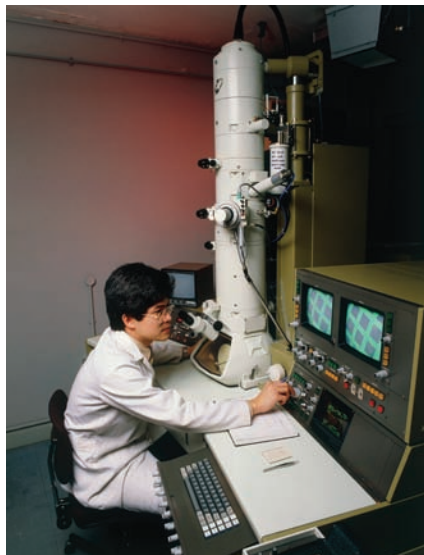
■ Figure 1.17 Using the transmission electron microscope
